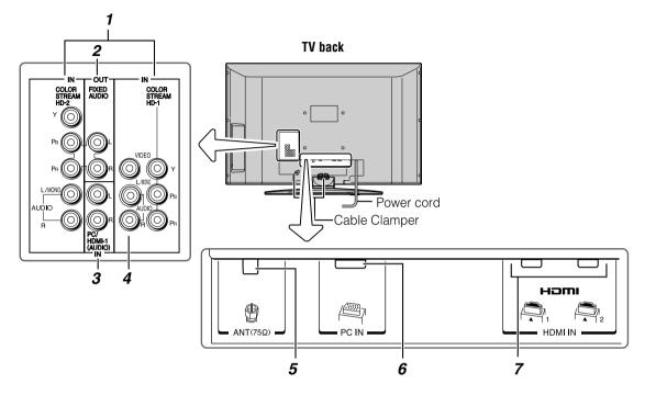
1 ColorStream<sup>®</sup> HD-1 and ColorStream<sup>®</sup> HD-2 — Two sets of ColorStream<sup>®</sup> high-definition component video inputs (with standard analog audio inputs) for connecting devices with component video output, such as a Toshiba DVD player with ColorStream<sup>®</sup>.
